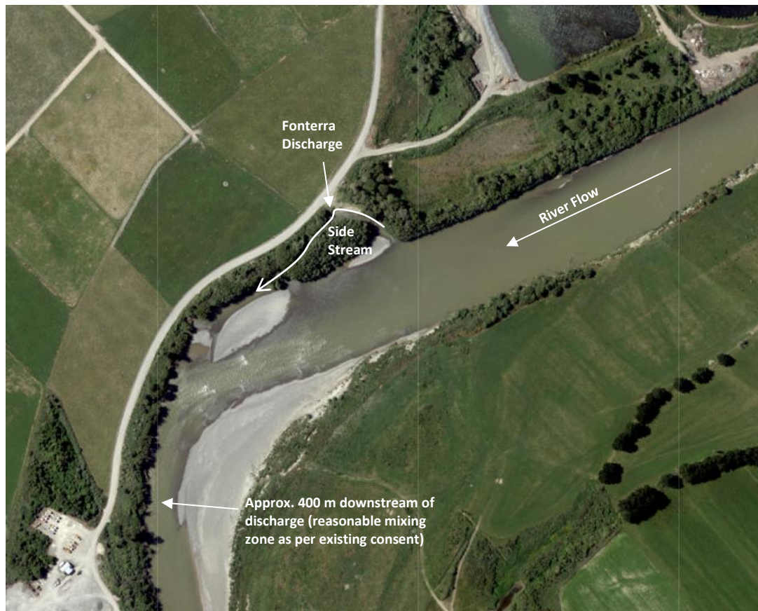
Figure 3.3: Close Up of Discharge Point to Manawatū River
